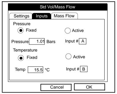
Figure 4-8: The Inputs Tab in the Standard Volume/Mass Flow Option
